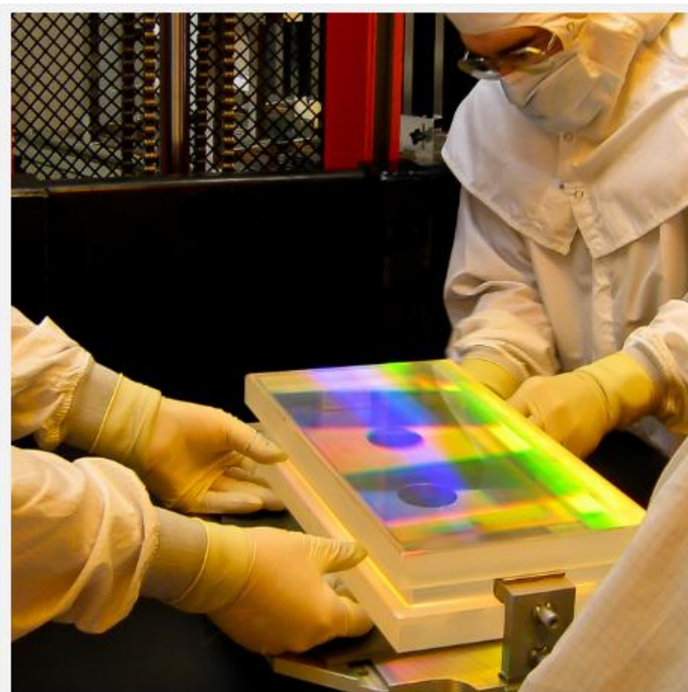
420 mm x 210 mm high-intensity laser MLD grating
