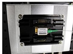
1550nm PM SLD Laser diode
